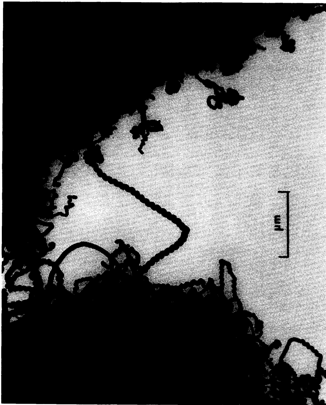
FIG. 7. Transmission electron micrograph showing the spiral form of filaments produced by Ni-Fe + TiO 2 catalyst particles after exposure to 2 Torr acetylene at 825°C.
