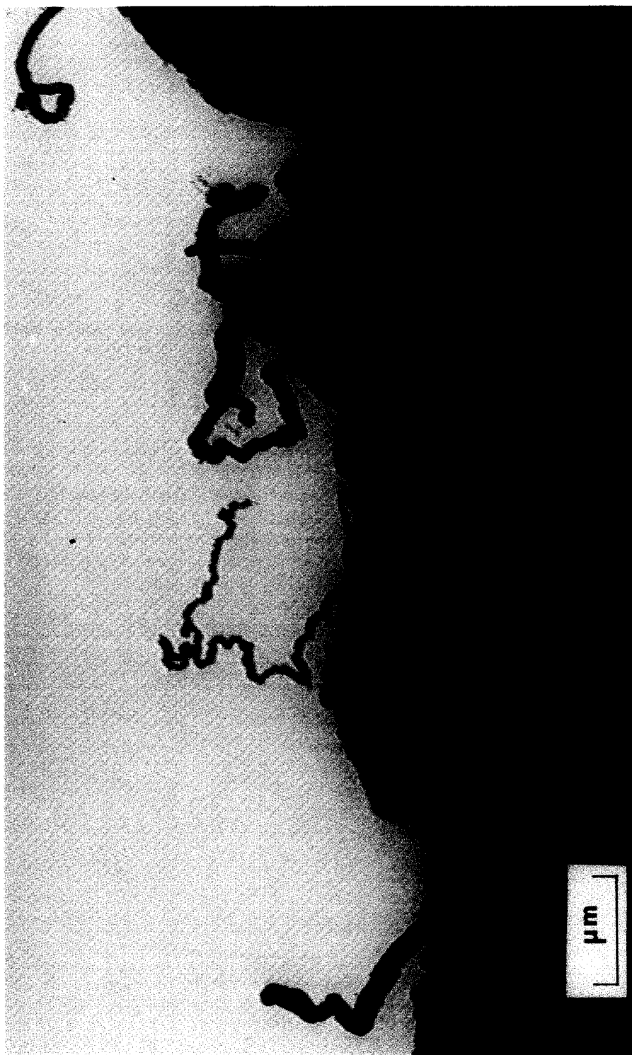
FIG. 3. Transmission electron micrograph showing the appearance of carbon filaments from Ni-Fe + SiO 2 /acetylene at 800°C.
